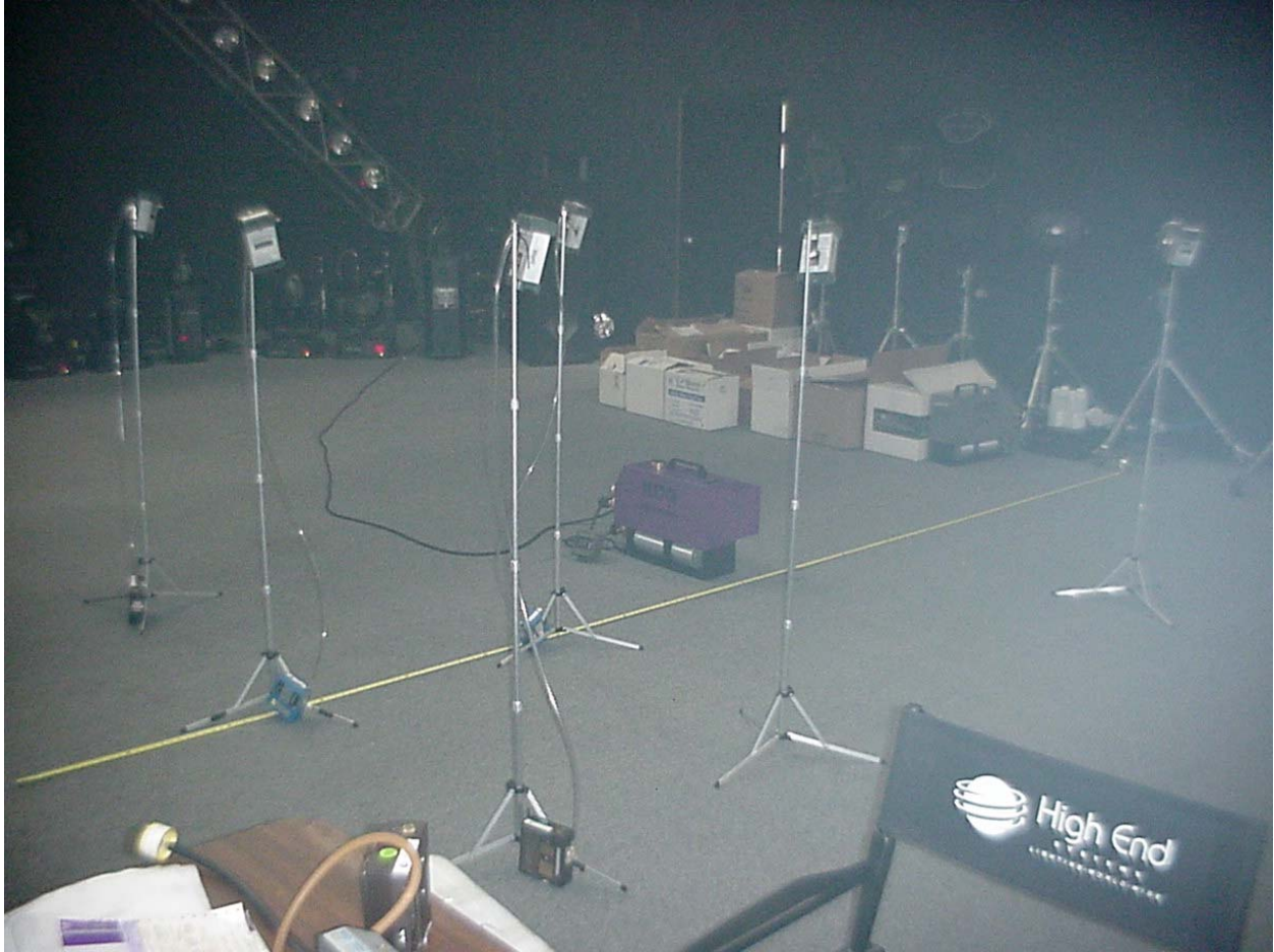
Figure 3. Example sampling configuration consisting of six sampling/monitoring tripods situated at three-foot intervals around a vertical-release hazer (center).
