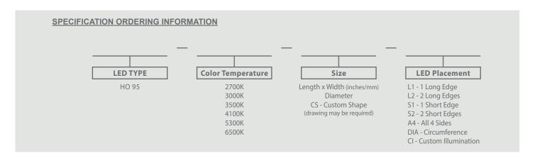
**HO 95 - 5300K - 12 in x 12 in - A4** specifies a 12 in square LitePad with a color temperature of 5300K and LEDs on all sides. **HO 95 - 2700K - 200 mm - DIA inside** specifies a 200 mm round LitePad with a color temperature of 2700K and LEDs on the inside circumference.
